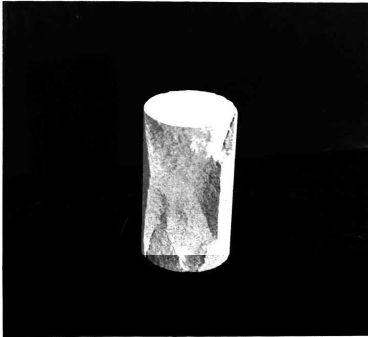
Figure 8. Photograph Showing The Fracture Pattern in a Limestone Specimen
