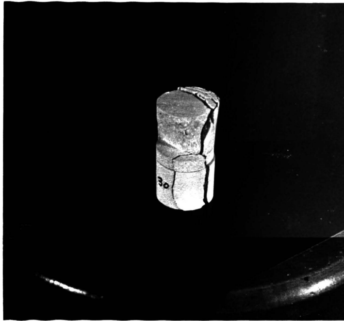
Figure 21. Photograph Showing the Fracture Pattern in a Three-Layered Specimen Having s:l:d=1:0.44:1 and With an 2:1 Length to Diameter Ratio
